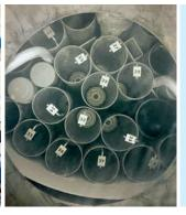
The MVE815 can hold 52 canisters for 67-70 mm goblets with either 2, 3 or 4 layers of straws
